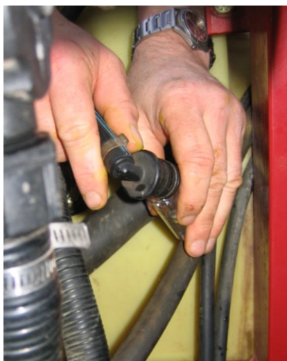
Photo 3. A sample from the valve with even pressure device is taken.
