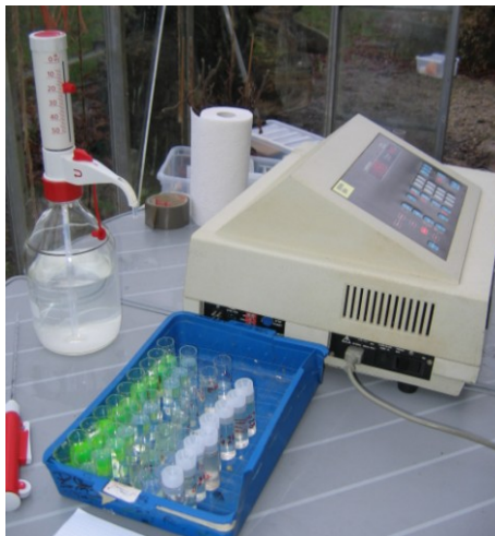
Photo 2. Samples with tracer are ready for analysis in the fluorimeter. The exact amount of tracer can be measured.
